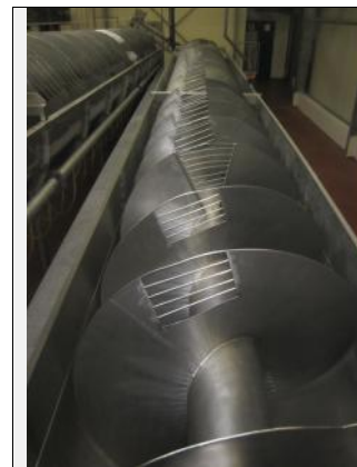
Figure 8 As your plant expands, you may run out of space unless you opt for wider chillers at the outset
