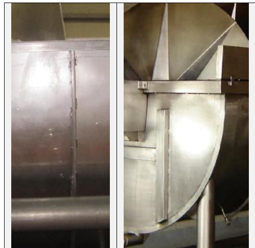
Figure 9 Flange-jointed sections and end-plates versus welded end-plates. Note also the tack-welded braces on the endplate. Tack-welding is not acceptable for machinery for the food processing industry. Furthermore if braces are added for strengthening the end-plate against buckling, they should be seam-welded or they will not work. Note yet again that the brace consists of an SS channel with both ends left open to allow debris to accumulate!
