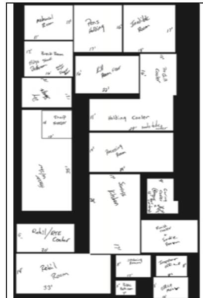
Figure 10 This picture 8 best illustrates the process of assembling blocks together to prepare both a plot plan and a process building layout.
